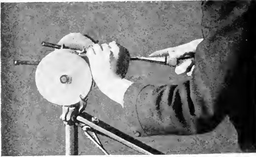
Fig. 21. Grinding a Chisel.
